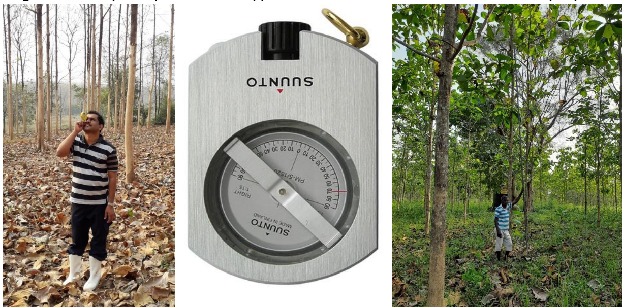
Figure 3: Total Tree height was measured by hypsometer and a pole, used instrument of sun unto meter is shown in above
